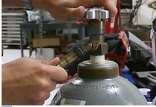
**1** Sensors were tested using laboratory gas specifically formulated to yield 11.76 AFR and 13.15 AFR. This way each sensor sees the exact same "exhaust gas", letting us measure the accuracy and responsiveness of each meter.
