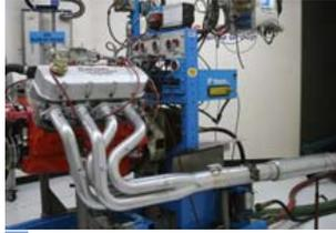
**2** After testing with lab gas the sensors were run-in for an hour with race fuel, on a test engine (Westech just happened to have a Chevy motor in the dyno room that day.) The run in simulates the wear and tear a sensor goes through with live fuel and heat conditions.
