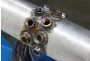
**3** Nine bungs were welded into the exhaust; eight for the sensors under test and one for Westech's own meter. Datalogging was performed during the engine run-in to assess the capabilities of each meter.
