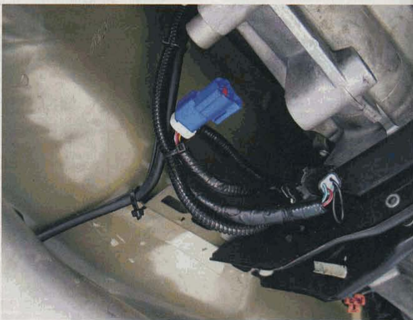
THE LC-1 wire harness was routed and secured out of the way, and fed up to the shifter boot.
