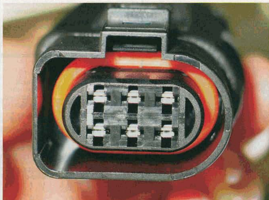
THE LC-1 Lambda cable features a weatherpack-style connection to keep out the elements, which is good considering most wide-band installations inhabit the underside of the vehicle.
