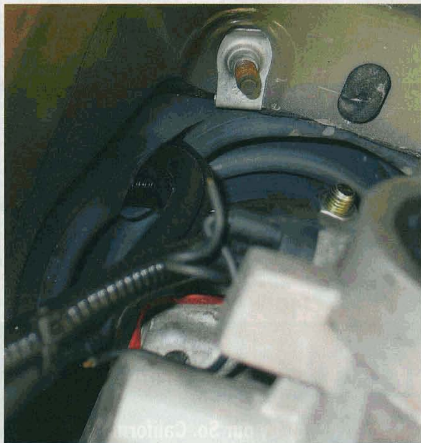
THE SHIFTER boot seemed as good a place as any to run the LC-1 harness through. The boots are easy and cheap to replace, and the rubber will protect the harness.
