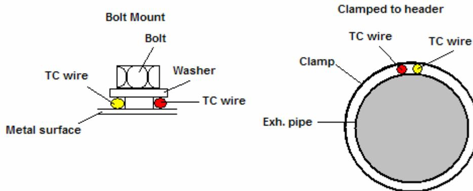
The TC-4 will work with either isolated or grounded junction thermocouples.
