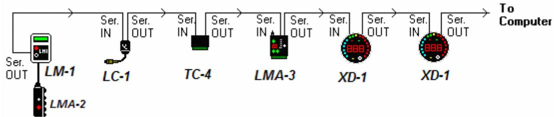
Devices attached to the LM-1's analog input count as being part of the LM-1's 6 channels. They don't count extra. XD-1's do not contribute any channels, so you can add as many as needed.
