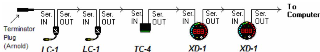
***Notice that the LC-1's are connected BEFORE the first TC-4. LC-1's should always be connected before the first non-LC-1 device (except if the first device is an LM-1).***
